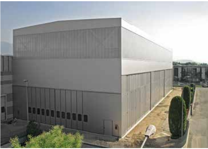
External view, folding door with double leaf packs 4+4, motorized, height of the hole 9000mm
