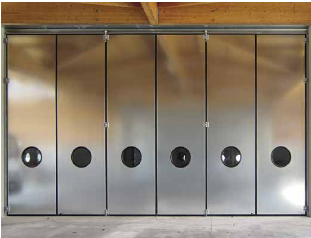
External view, folding door with double leaf packs 3+3, without track on floor, leaves made of galvanized steel, with portholes
