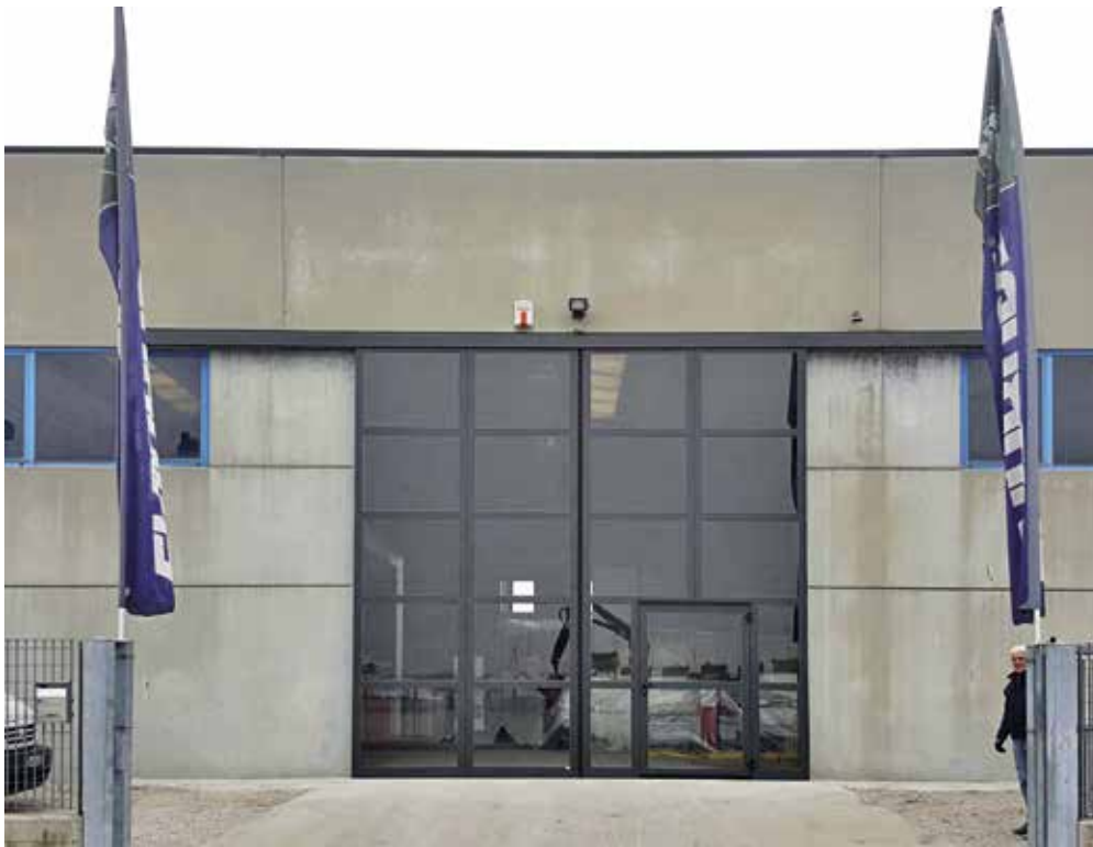
External view, sliding door with two leaves, with pedestrian door with lowered obstacle
