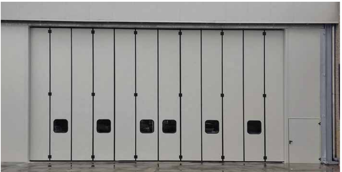
External view, folding door with double leaf packs 6+6, with side fixed panels, height of the hole 6500mm
