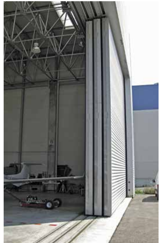
Sliding doors with overlapping leaves, with track on floor, motorized, height of the hole 7000 mm
