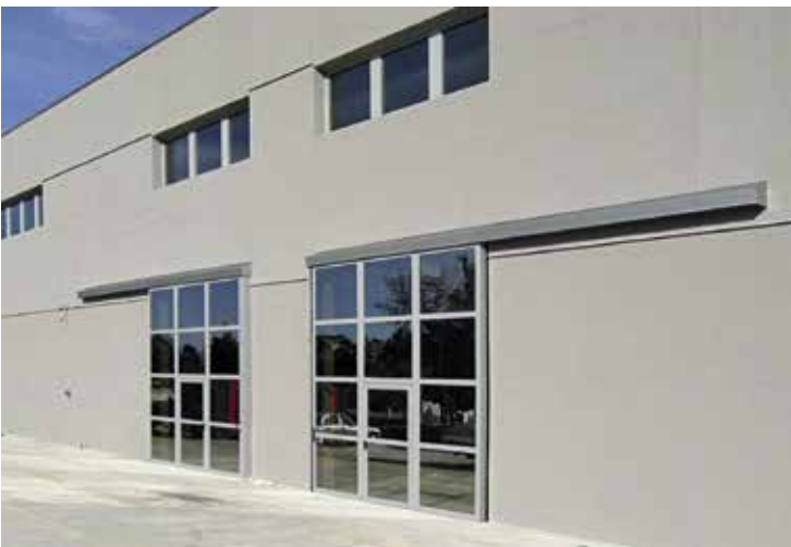
External view, sliding door with single leaf, with pedestrian door with lowered obstacle
